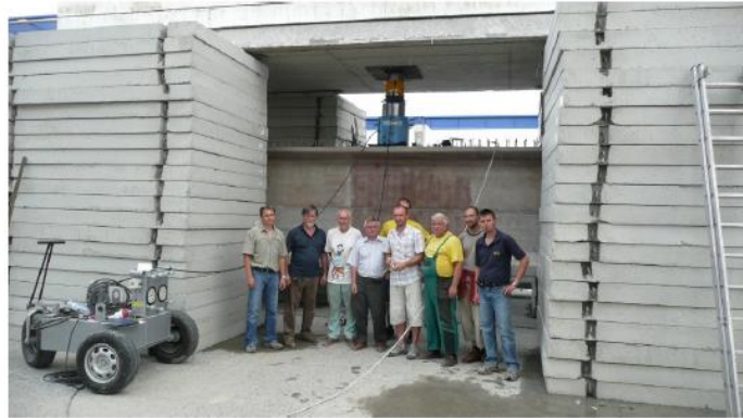
Bridge beam certification – static load tests
