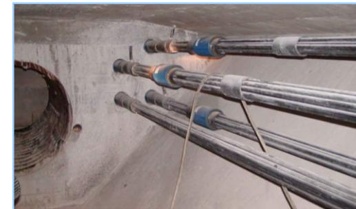
Monitoring of forces on corroded strands during prestressing
